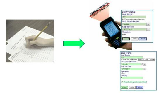
SPTS is designed for use by shop-floor workers who have limited computer literacy. By using barcode scanning manual data entry is minimized. Also SPTS warns users if they make a data collection mistake and allows immediate data correction. SPTS only captures the minimum data needed for each tracking situation. This minimizes training time and eases the introduction of data collection technology to the shop floor.
