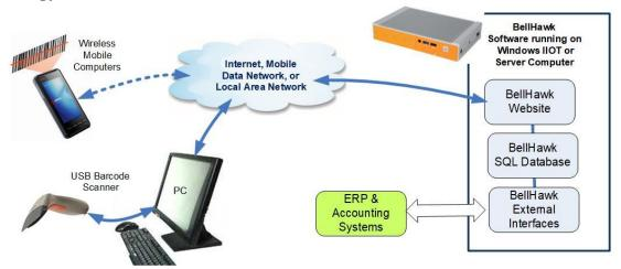
The BellHawk JTS data collection software consists of a specialized website and a SQL Server database that run on a Windows Server IIOT or Windows Server computer. All user interaction is performed using web-browser based devices thereby avoiding the need to install custom software in each data capture or viewing device.
