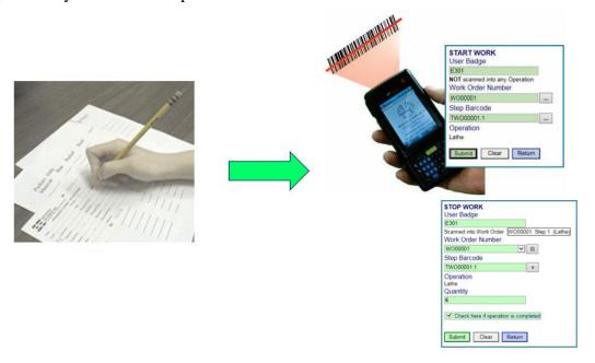
JTS is designed for use by shop-floor workers who have limited computer literacy. By using barcode scanning manual data entry is minimized. Also, JTS warns users if they make a data collection mistake and allows immediate data correction. JTS only captures the minimum data needed for each tracking situation. This minimizes training time and eases the introduction of data collection technology to the shop floor.
