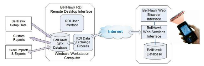
The RDI software uses the free Microsoft SQL Server Express database server to create and maintain a copy of selected tables within the BellHawk database on a local data exchange database (DEX) on a user's desktop PC. Users can then use Excel to create their own exports from this database or can use third party reporting software, or programs written in a language such as Python, to generate their own custom reports from the DEX database.
