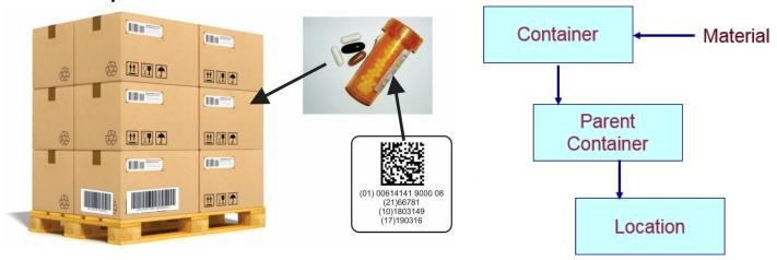
Unlike accounting systems, which track the quantity of material in stock, BellHawk tracks material in containers. At its core it is tracking the quantity of each item in or on each container, such as a box, barrel, or pallet. To compute the inventory of a specific item, BellHawk adds up the quantities of the item in all the containers.
