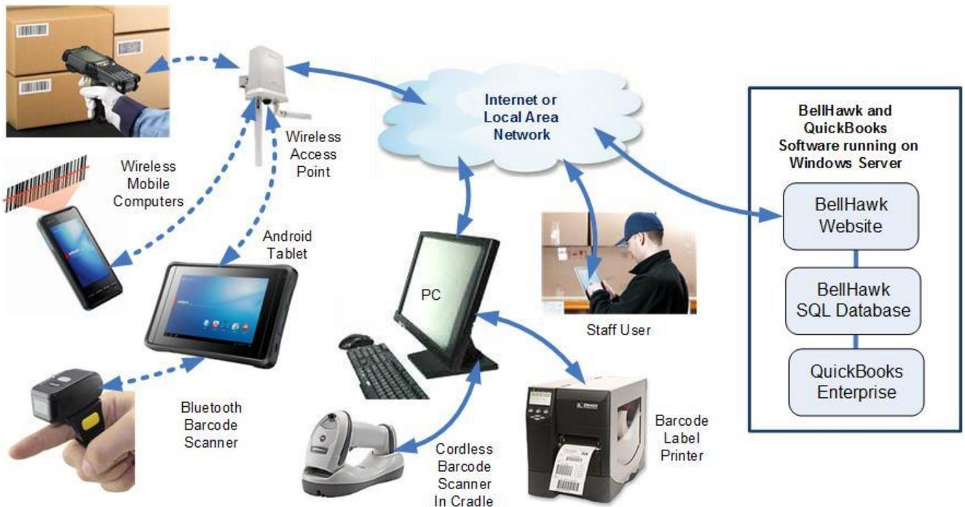
QBITS uses a web-browser interface that is simple for material handlers to use with a wide range of mobile devices including Android tablets with external Bluetooth barcode scanners and ruggedized mobile computers with integral barcode scanners. This includes the use of wearable finger-mounted barcode scanners for hands-free scanning. QBITS can also be used with fork-lift truck mounted barcode tracking systems which use touch screens as well as with fixed station PCs and tablets.
