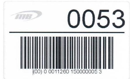
After these SSCC barcode labels are attached to the cartons, the labels are scanned using ruggedized wireless mobile computers (with integral barcode scanners) to record each container into inventory. As part of this activity, the Bellhawk FMS automatically associates the data that was previously associated with the label (when it was printed) to the container to which it is now attached.
